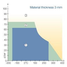
As the maximum operating pressure and load bearing capability are both depending on the gasket thickness, KLINGER provides thickness related pT diagrams.
