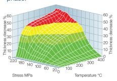
The diagram shows the additional thickness decrease at temperature.
